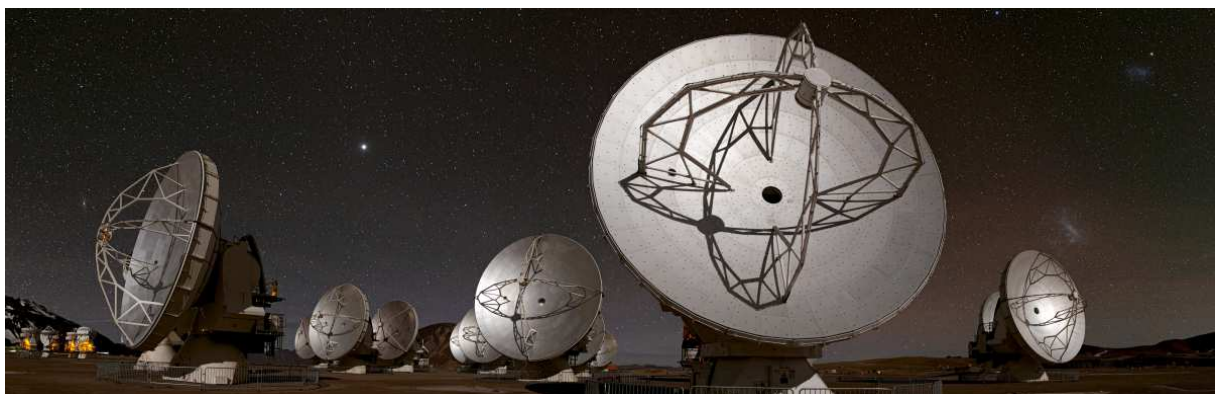
FIGURE 10 – Fifty-four 12-metre and twelve smaller 7-metre dish antennas of the ALMA array work together as a single telescope. Each antenna collects radiation coming from space and focuses it onto a receiver. The 66 ALMA antennas can be arranged in different configurations, where the maximum distance between antennas can vary from 150 metres to 16 kilometres. ©ALMA (ESO/NAOJ/NRAO)
