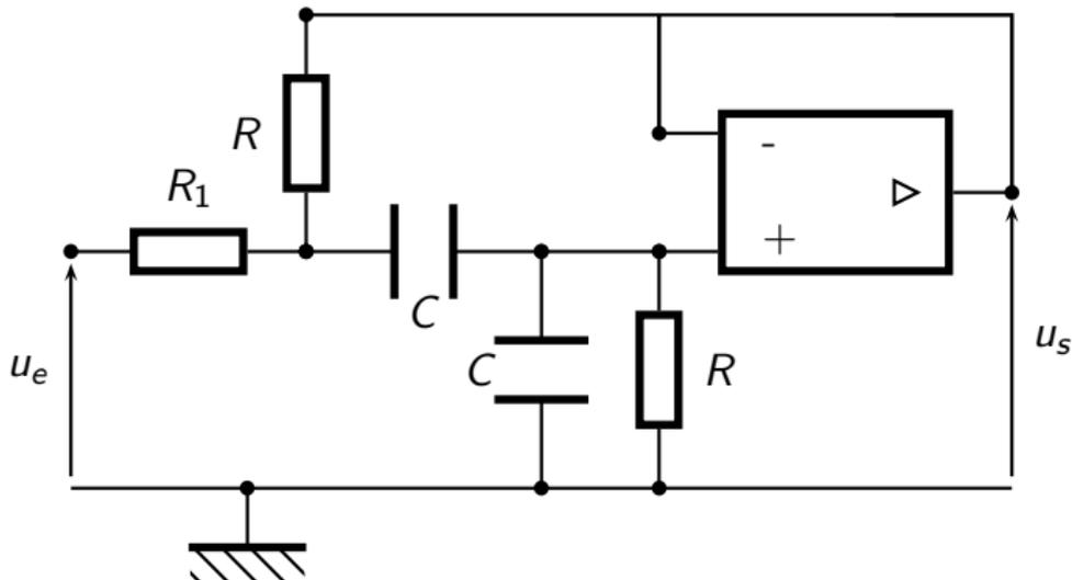
$$\underline{H}(j\omega) = \frac{H_0}{1 + jQ \left( \frac{\omega}{\omega_0} - \frac{\omega_0}{\omega} \right)}$$
