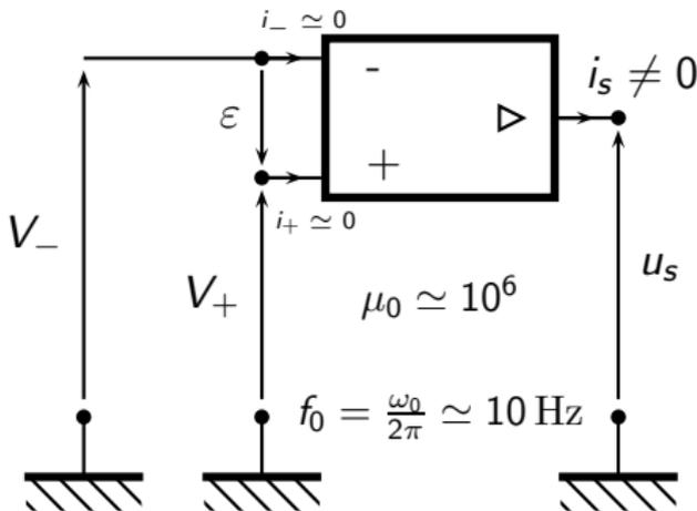
$$\text{Régime linéaire : } u_s = \underline{\mu} \varepsilon = \underline{\mu} (V_+ - V_-) = \frac{\mu_0}{1 + j \frac{\omega}{\omega_0}} \varepsilon$$
